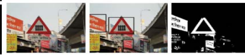
(a) Original image (b) Signs detected (c) Color segmentation
