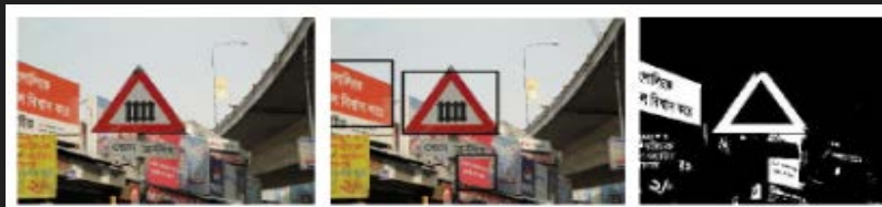
(a) Original image (b) Signs detected (c) Color segmentation
